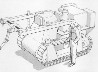
MOBILE REMOTE HANDLER, pictured here, and a remotely operated overhead crane system, will be used to move irradiated materials in the "hot room" of the SERF. Heavy lead shielding around the handler will protect an operator from harmful radiation. personnel against radiation exposure.
